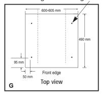
Position the base into the recess with its front edge as far forward as the adjoining plinth line will allow. The reason for placing the base in this position is to allow a small strip of beading to be fitted in front of the appliance feet.
